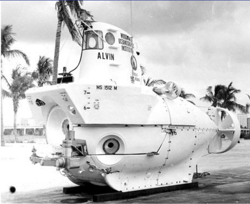
Deep ocean submersibles developed from the bathyscaphe to be more maneuverable. The first of these, *Alvin*, was built in 1964 and so far has made more than 4,200 dives. Alvin is well known for exploring newly discovered hydrothermal vents in the 1970s. It also took scientists down to survey the deep-ocean wreck site of RMS *Titanic* in 1986.
